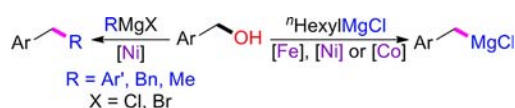
Scheme 1. Catalytic Transformations of Benzyl Alcohols with Different Grignard Reagents via Fe-, Ni-, or Co-Catalyzed sp^3 C–O Bond Activation
